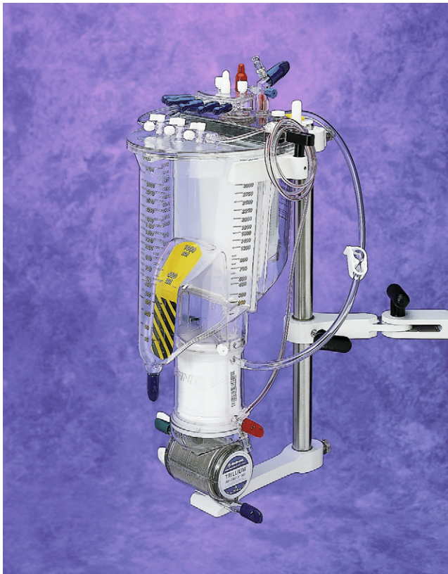
FIGURE II.5.13 The Medtronic Affinity® oxygenator with integral heat exchanger and attached hard shell blood reservoir. Note the mesh filter within the reservoir to prevent passage of macroemboli through the heat exchanger and oxygenator. (Image courtesy of Medtronic, Inc., Minneapolis, MN.)
