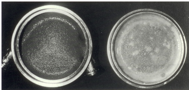
FIGURE D.4 Pseudointima developed on the interior textured surfaces of the HeartMate VAD after an implantation period of 243 days. On the left is the titanium surface with sintered microspheres and on the right is the textured polyurethane surface. (Reprinted from Poirier, V. L. (1999). Thorac Cardiovasc Surg 47 (suppl), 316–320.)
