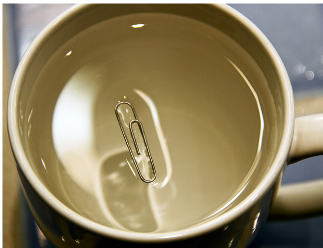
FIGURE I.1.6.2 A metal paper clip floats on the water surface “skin,” a manifestation of water’s high surface tension. (Photograph by Buddy Ratner.)
